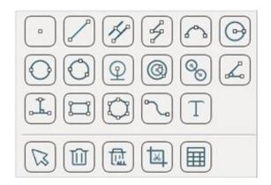
Point: Move the mouse pointer to the position to be measured, click the left mouse button and raise it to complete the drawing and display the corresponding coordinates.
