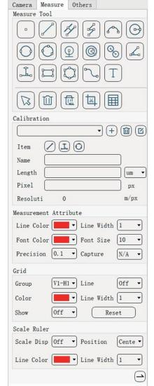
*Note*: The coordinate values change depending on the position of the scale and the size of the calibration.
