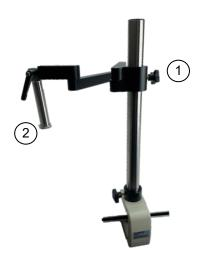
Insert the movable arm into the microscope column and tighten the locking screw (1). Now loosen the knurled screw (2) and insert the holder for the microscope head into the shaft.
