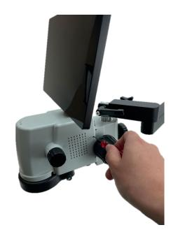
To attach the microscope head to the stand, tighten the screws (2x) on the outside of the housing using the Allen key supplied.
