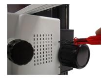
To attach the microscope head to the stand, tighten the screws (2x) on the outside of the housing using the Allen key supplied.
